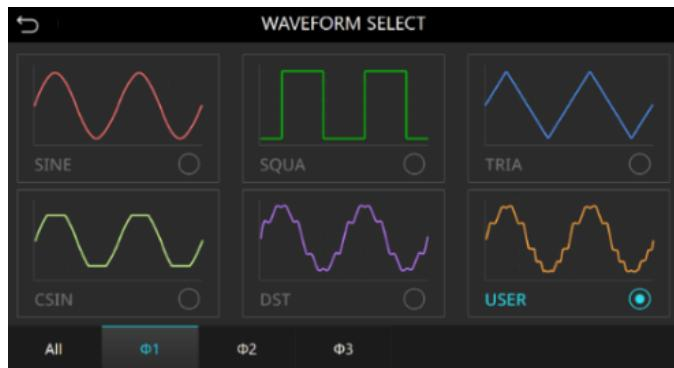
testing under atypical or extreme power quality conditions. With independent multi-phase configuration, different custom waveforms can be assigned to  $\Phi 1$ ,  $\Phi 2$ , and  $\Phi 3$ .
